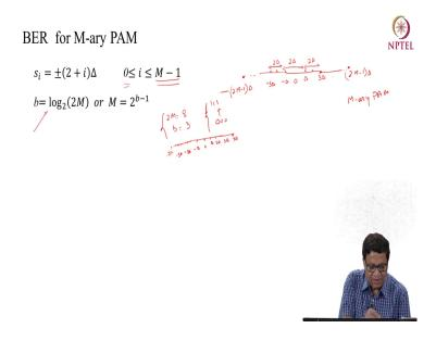
So, we will try to calculate for a generic system which is M-ary PAM system. So, let me draw the constellation of a M-ary PAM system it will be. So, say this is 0 and say this is delta, which is away delta point of delta distance away and this is say minus delta. So, this whole thing between two constellation points the spacing is 2 delta. The next will be at 3 delta.
