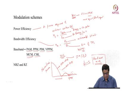
So, for example, if I plot the normalized power on this side, normalized power and this side is say normalized frequency. So, for NRZ, this is the power spectral density for NRZ. So, this is you can say on off keying NRZ OOK on off keying NRZ. And for on off keying RZ, I am drawing with a dash and this will be 0 here.
