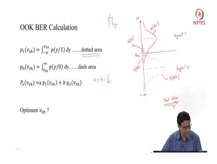
Now, let us take a simple on off keying system and try to calculate the BER for such a system. So, as I mentioned on off keying is you have this is a digital pulse and you modulate your LED or laser diode. So, whenever there is one, the LED is forward biased and emits power, whenever it is 0, there is no power coming. So, basically you are getting on off the device and off of the device, there is on off keying.
