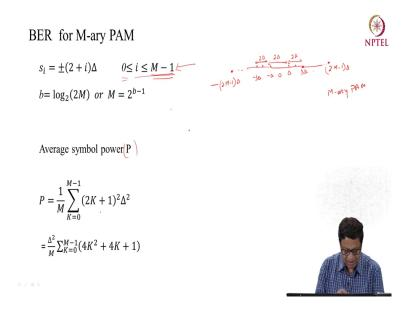
So, now let us try to calculate the BER for a such a system. So, the average symbol power if I want to calculate the average symbol power because each will have you know different power levels. So, the average symbol power will be given by 1 by M this is a total number of levels summation K is equal to 0 M minus 1 2K plus 1 whole square delta square. So, this is the average powers for example, if K is equal to 0. So, this becomes delta square.
