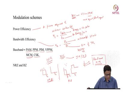
Now, in systems which are based on light for example, visible light system normally they use LED or laser as the source and these source they require positive signal and real signals. This
