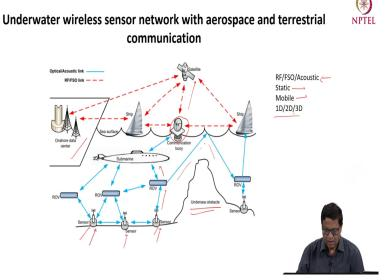
So, these are some of the applications of underwater communication as you see in this diagram. The red lines are either RF link or free space optics link or optical wireless link and the sky blue line is actually communication using either optical communication or acoustic link.
