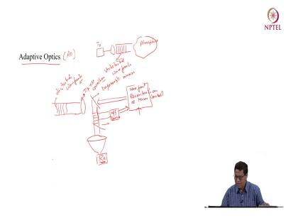
So, this is one method and the third method is use of adaptive optics which is also called as AO. So, in adaptive optics what happens actually there is a undistorted wave front at the transmitter. So, let me first make the diagram. So, this is for example, T x and you have this is a some sort of lens and you have undistorted wave front which is going to the atmosphere. So, this is the you know atmosphere part and these are undistorted wave front wave fronts and distorted wave fronts.
