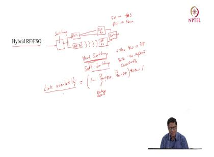
Another method which can be used for mitigating the atmospheric turbulence is use of both RF and FSO. So, in normally what is done here, you have the input stream and then this is a switching block or switching at the transmitter switching at the transmitter. So, this is switching and then you have two systems one is FSO transmitter the other one is RF transmitter.
