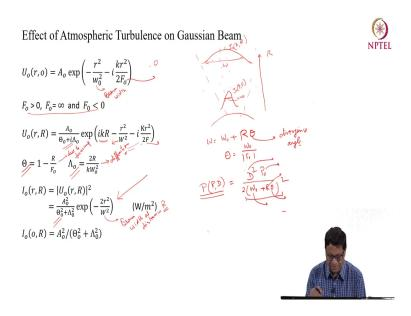
So, as you suppose this is your input Gaussian Beam and this is given by say beam width omega 0 and as it travels a distance R. So, this beam will actually spread and this will become omega that is the distance of R it has the beam width has become omega and so this is the I 0 r, R and this was I 0 E 0.
