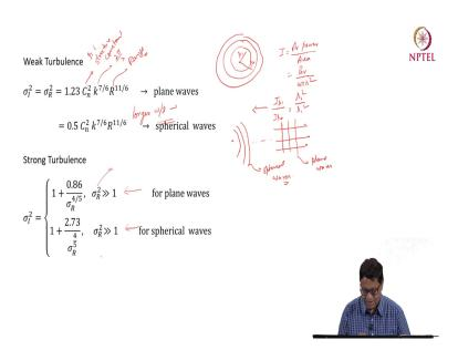
So, there are 2 types of waves plane waves and the spherical waves. So, this scintillation index has been defined both for plane waves and spherical waves. So, when you have a source and it is emitting in all the directions. So, this is say for example, r 1 this could be r 2 let me write a bigger. So, this is say r 1 this could be r 2.
