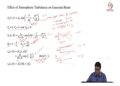
So, Gaussian Beam can be represented by say U r at r is equal to 0 this is capital R that is initially a 0, A 0 is the amplitude exponential minus r square this is the beam width minus ik r square k is the wave number and F naught is given by is a F naught is a phase front radius of curvature phase front radius of curvatures, that depends how your beam forming.
