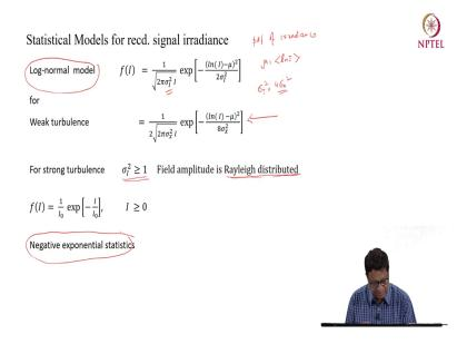
So, now let us go to the some of the Statistical models for received signal irradiance. So, there are some well-known models which are defined how the which actually tells about the PDF of the irradiance which is received which is received irradiance at the receiver.
