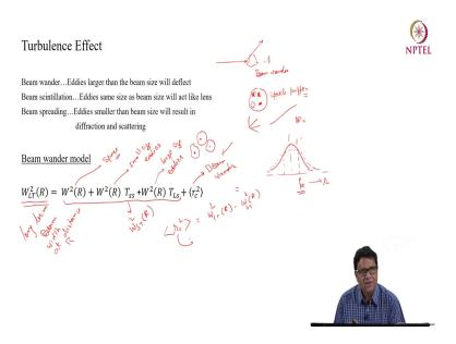
So, let me again explain this; so, you have hot spot moving and also the centroid of the beam is also moving around its central position. And because of this the long term effect will be a bigger you know hot beam size or spot size of dimension W L T. And this W S T is for the smaller because of the hot spots and then this gives you the beam wander part which is and the whole beam wander model can be modeled by this equation.
