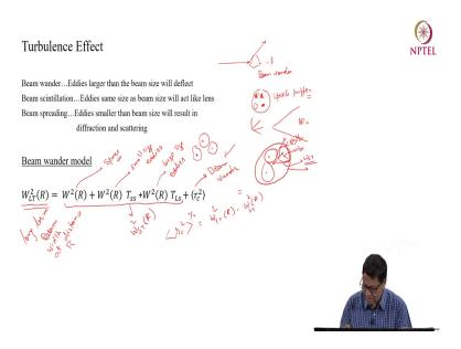
So, now let us see the effect of turbulence, what actually happens because of turbulence? So, the first effect which happens is beam wander. Now, there are eddies which are small which are size and then you have a beam size. So, if the eddy size is larger than the beam size, then the whole beam is actually deflected and in the receiver there is a possibility that you might miss the beam.
