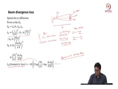
So, let us try to understand this beam divergence loss. So, beam divergence loss and let us assume that there is a transmitter here and I am this is a the transmit optics here. So, this will
