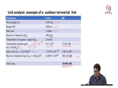
So, this is a example of a terrestrial link where I have considered 1 wavelength which is 15 nanometers this is same as used in optical fiber communication system. The distance which I am referring is 1 kilometer and I am interested in transporting or transmitting 1 gigabits per
