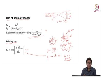
So, sometimes one can use a beam expander. So, beam expander actually say 2 lens system. So, you have for example, this is a source and it is emitting like this. And then you have a first lens here it converges a light here and then you have another lens which will you know collimate the beam.
