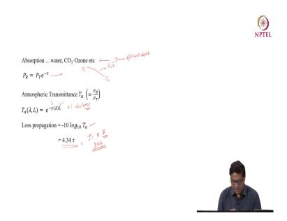
So, absorption because in the atmosphere you have water molecules or carbon dioxide or ozone, so they basically absorb the light so, the light which is received, the intensity or the power gets reduced because this is the absorption. Let us also now understand as it travels, how can we model the light traveling from transmitter receiver.
