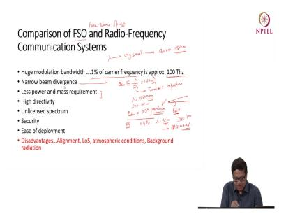
So, let us now briefly understand a comparison between a free space optics. This FSO is Free Space Optics and radio frequency communication system. So, the basic difference which comes from the fact that the wavelength of optical channel is very very small; it is very small as compared to RF channel, as we have seen in traditional systems the wavelength is of the order of you know 1300 nanometers or 15, 50 nanometers, right.
