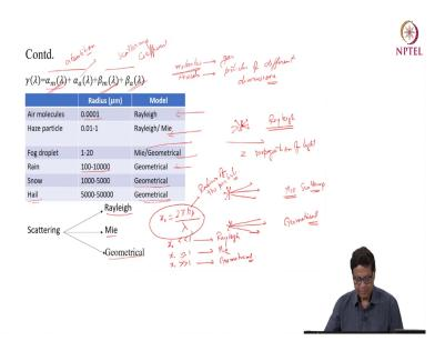
So, now let us understand this gamma lambda. What are the different components of attenuation coefficient? So, it has actually the attenuation happens because of molecules in the atmosphere or the aerosols. These are you know gas gases, they are present in the
