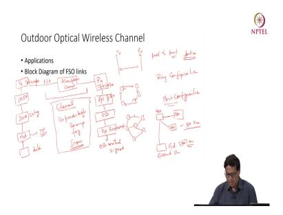
So, first let us try to understand, what are the different applications of outdoor optical wireless channel. So, first to the immediate application can be you know connecting two points. This is T x, this is R x, suppose you are not able to lay fibers here or it is difficult to lay fiber. For
