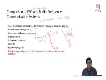
So, in that case, so suppose you have a laser beam and this is your Earth and this is your say Mars. And then you suppose you have a optical beam here and then the divergence which it has traveling from Mars to Earth is actually 0.1 of the Earth diameter 0.1 of the Earth diameter. Whereas, if you see for example, in RF case this is Mars, this is Earth. So, this will diverge much more and this is distances of the order of say 100 times earth diameter.
