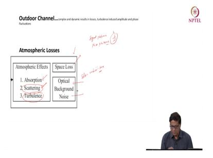
So, outdoor channel as I mentioned is quite complex and dynamic. It is changing with time. So, and it will result in losses, there will be a space loss as the light travels from one place to another place. And there is a turbulence in the atmosphere and this turbulence will actually induced variation in the amplitude, variation in the phase which is actually noise.
