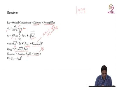
Let us now understand receiver and then we will see the you know how channel can be modeled. So, receiver I am assuming that there is a optical concentrator and which may have a gain of one and then there is a detector and there is a preamplifier which amplifies the signal and then it is given for further processing. So, assuming this is the receiver collection area, then this is the photo diode area once you are using a concentrator.
