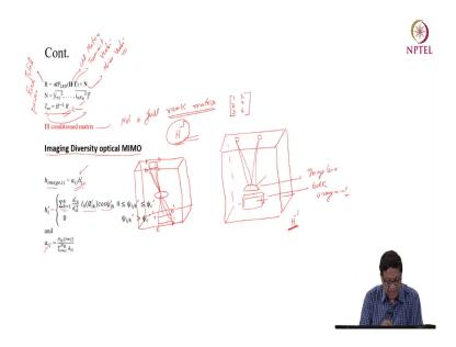
So, R total power this is the total power total received power is responsibility into P LED into H T. So, these are two matrix, this is H is a channel matrix and this is your transmit vector, this is your noise vector noise vector because there are many receivers; so, it will be a vector again.
