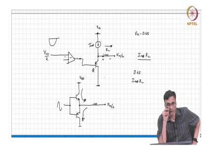
So, what is the maximum swing? So, the voltage across the maximum positive voltage across the  $R_L$  is basically  $I_{ref}$   $R_L$ , ok. So, what do we see? What is the model of the story? So, in the NPN case the upper limit is  $V_{CC}$  - 0.65 which is independent of  $R_L$ , the lower limit is dependent on  $R_L$ . In the PNP case, the lower limit is independent of  $R_L$  the upper limit is dependent on  $R_L$ , right. What do we want?
