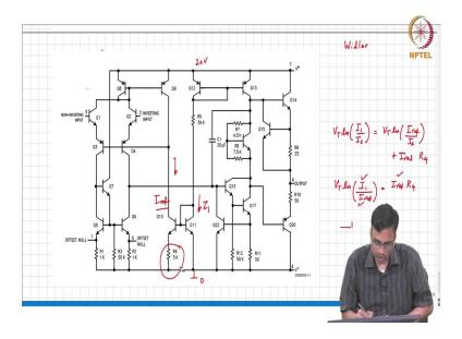
So, you want this current to be, you know, largely independent of the supply voltage, ok. So, basically the idea is that if this current is let us call this  $I_1$  and you know how do we get  $I_{ref}$  here? What do I mean? How do we find out what  $I_{ref}$  is? Well  $V_T \ln(I_1/I_S)$  must be equal to  $V_T \ln(I_{ref}/I_S) + I_{ref} R_4$ , correct. So, basically this means that this  $V_T \ln(I_1/I_{ref})$  must be equal to  $I_{ref} R_4$ , ok.
