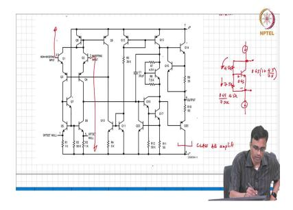
This is 7.5 K, this is 4 and a half K. So, what is this voltage? Some current is flowing. So, what is the voltage here base emitter voltage? 0.65. So, what is the current flowing here? 0.65/7.5 K what is the voltage across the 4.5 K? So, what is the voltage drop you see there? 0.65 (1 + 4.5/7.5), right.
