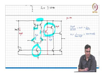
So, basically, the second stage has to be going to load the first stage, and therefore, we need a VCVS, and for the active load, we simply short the base and the collector, right? So, in other words, the collector potential must be the same as the base potential, right? But so, I mean so, in principle, you know, we could have shorted the collector and the base of Q5, but you know, soon it will become apparent why Q7 is there, right?
