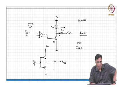
But, when the input is 0, what happens? I mean in other words when the input is  $V_{CC}/2$  what happens? No current flows because basically the you know if this is  $V_{CC}/2$  and this is  $V_{CC}/2$ , both the transistors are off because the  $V_{BE}$  is 0, correct?
