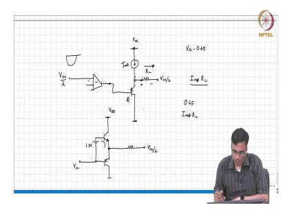
So, what do you know? What should be done is you have you know there are many ways of doing this you know one way is to put a battery off exactly 1.3 volts, ok. So, and you know perhaps put you know V in here. So, both the transistors are at the verge of conducting if the input goes slightly positive, then the NPN transistor will conduct immediately when the input
