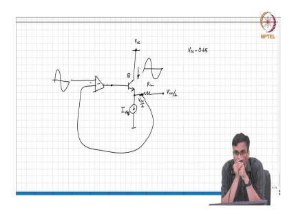
Maybe ok let me remember the load is connected to analog ground which is  $V_{CC}/2$  this is  $V_{CC}$  under quiescent circumstances this voltage is  $V_{CC}/2$ . This is  $R_L$ , correct? When you apply a signal, you know the output voltage is swinging like this. What is the maximum voltage that the output can go before something bad happens to the devices? If the output voltage keeps going high what happens eventually to the transistor?
