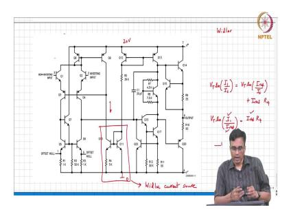
So, this is one way, this is what this current source is called the Widlar current source ok. And, is a clever trick to get a small current while still using a small resistance ok. And, what comment can we make about the supply sensitivity of this current? This current is actually sensitive to supply, but the voltage across you know voltage across the base of between the base and emitter of Q11 is largely independent because it is logarithmically you know the base emitter voltage is ln(I).
