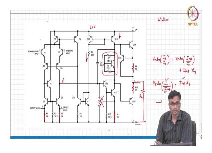
And, so, the output basically is you know through some load resistance is  $R_L$  which is outside the chip. So, you know again for the time being these resistors 25 ohms and all that you and 50 ohms lets neglect, ok. We will add we will figure out why they are needed, you know just a little bit. So, Q14 how does that behave? It is a common collector stage, right.
