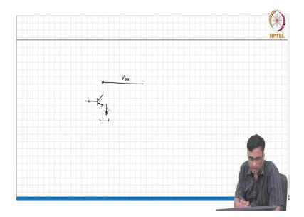
So, basically, the root cause is the fact that we are taking what the transistor is doing, which is basically converting this voltage to a current and pushing that current through a resistor, right? So, the root cause of the problem is the fact that we are taking the output at the collector, correct?
