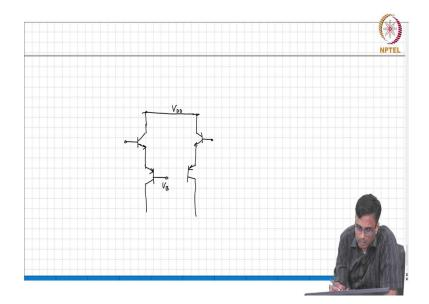
If you want a current source, In other words, when you are looking at the collector, what is the output resistance looking like here? When the source is grounded, what is the incremental impedance looking into the collector when the transistor is active? It behaves like a voltage-control current source because the output impedance is infinite, which is correct.
