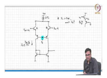
So, we want to find the sum of the currents quiescent currents in transistors Q1 and Q2 and tweak the base voltage, so that the sum of the currents always remains constant right equal to some reference current. So, where can we find the sum? Is there some way of finding where you can put an emitter to find the sum of the two currents in the transistor of, I mean the sum of  $IQ_1 + IQ_2$ ? What do you think we can do? Where can we measure? Ok so, a good place to measure is the collector.
