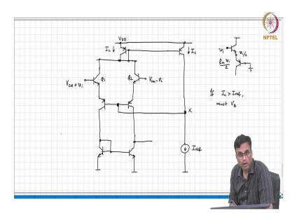
Use KCL to compare, but so, basically you make. So, one way of doing this is to make a copy of this current. How do you make a copy? Current mirror, right. So, this is the current mirror, ok and then you will compare this with  $I_{ref}$ . So, this is  $I_C$ , this is also  $I_C$  ok. So, this is  $I_{ref}$  if  $I_C$  is greater than  $I_{ref}$  we must increase  $V_B$  for what happens to this node x?
