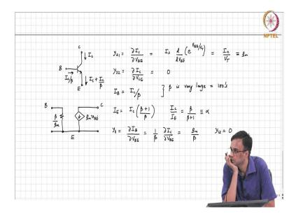
So, now that we have done this, the next thing to do is basically figure out what these device equations are. The next thing to do is figure out what the small signal models for the transistor are. And again, once you ensure that the transistor is operating in the active region, then as usual we will go and figure out what the incremental y matrix is.
