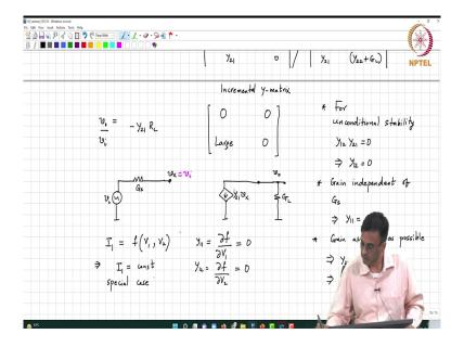
So far, we have taken some two port and then found the formula for its incremental Y parameters. Now we are trying to figure out what the characteristics of the device must be, of that box must be, the IV characteristics must be, so that the incremental parameters look like this. Does it make sense, right?
