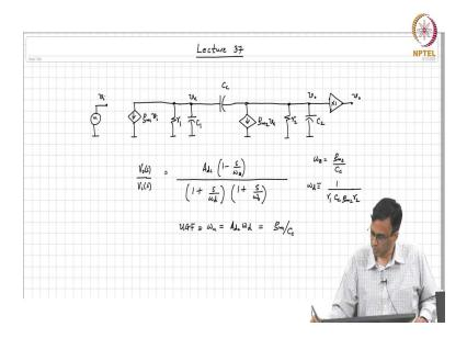
So, in the last class we were winding up looking at the frequency response of the 2 Stage Operational Amplifier and this is the small signal equivalent. So, this is the first stage  $g_m v_i$  goes into resistance  $r_1$  which denotes the total output resistance. For the first stage then there is a parasitic capacitance  $C_1$ , this is the dominant pole compensating capacitor, this is the transconductance of the second stage, I call that  $v_x$  this is  $g_{m2} vx$ .
