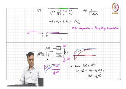
And we woke up yesterday. We were basically looking at the poles positions of the uncompensated system, right. Remember that the two poles of the uncompensated system are close to each other, right? And so, let us call them  $P_1$  and  $P_2$  and after the Miller capacitor is added, one pole moves very close to the origin, the other one moves further away. So, this is basically you can see that the poles are split. So, Miller compensation is also often called pole splitting compensation.
