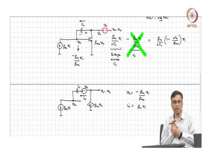
This is nothing but a current source which is  $g_{m2} v_x$ . So, if you have a voltage source in series with the current source, what is the effect of the voltage source? What does the voltage source do? Nothing.
