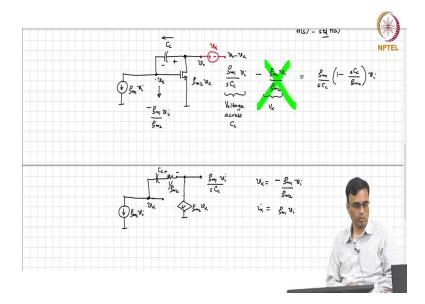
I mean, this gives you, I mean, this is a negative voltage, right. This is the same  $v_x$  in the opposite direction, right. So, the output voltage is basically  $v_x + 1/s$  C -  $v_x$ . So, the effect of  $v_x$  is canceled and therefore, you basically end up with  $g_{m1}/s$  C<sub>c</sub>.
