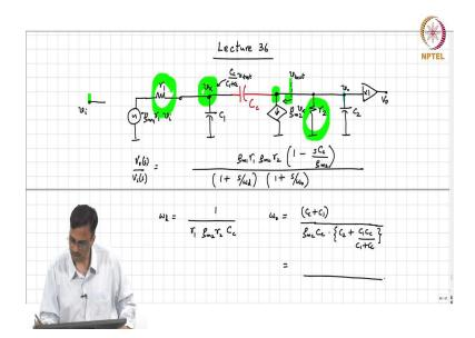
In the last class we were looking at the frequency response of a 2-stage operational amplifier. This was the small signal equivalent and we said that  $V_o$  by  $V_i$  is nothing but the DC gain. What is the DC gain? It is  $g_{m1}$   $r_1$   $g_{m2}$   $r_2$  is the right half plane 0 which is  $sC_c$  /  $g_{m2}$ . And this is the 2 poles are widely separated and there is a dominant pole and there is a what did we call the second pole?
