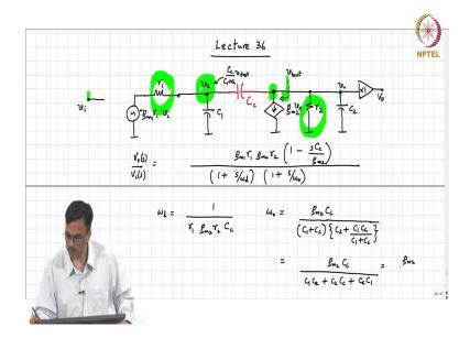
This is  $g_m g_{m2} C_c / (C_1 + C_c) (C_2 + (C_1 C_c / C_1 + C_c))$ . And consequently, this basically is  $g_{m2} C_c / (C_1 C_2 + C_2 C_c + C_c C_1)$ .
