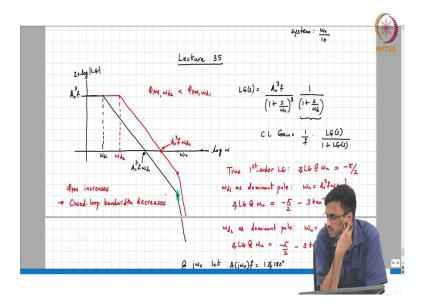
So, in this particular example, the phase margin where  $\omega_{d2}$  is less than the phase margin for choosing  $\omega_{d1}$ . So, phase margin is smaller, basically means that the margin you have for stability is smaller which means it's closer to be unstable. But what is it that you are gaining when you sacrifice phase margin? What are you gaining?
