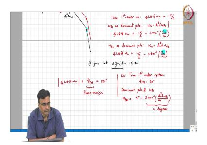
So, the system definitely becomes unstable with the angle of with a loop gain being  $180^{\circ}$ . The angle of the loop gain remains, becoming  $180^{\circ}$  when the magnitude is 1. So, in other words if you want to look at how far is this negative feedback loop from the edge of stability. What one can think of is how much phase so, the angle of the loop gain at  $\omega_u$ .
