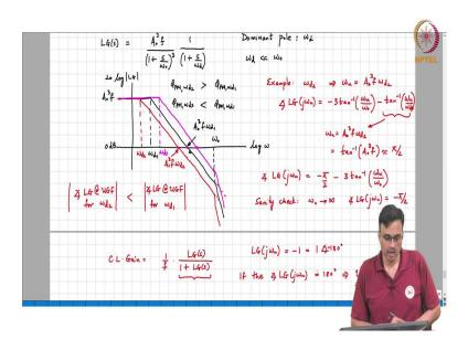
So,  $\phi_{pm}$  for  $\omega_{d2}$  versus  $\phi_{pm}$  for  $\omega_{d1}$ , which is greater? Which is the choice of dominant pole frequency  $\omega_{d1}$   $\omega_{d2}$  which of them has got a larger phase margin?
