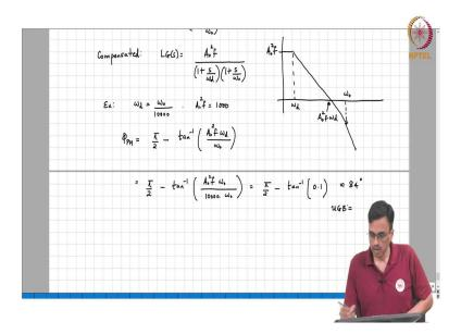
Is  $90^{\circ}$  -  $tan^{-1}$ ? So, what is the unit gain frequency in relation to  $\omega_o$ ? It is  $A_o^2$  f  $\omega_d/\omega_o$  which is nothing but  $\pi/2$  -  $tan^{-1}$   $A_o^2$  f  $\omega_d$  is what?  $A_o^2$  f  $\omega_d$  is  $\omega_o/10000$   $\omega_o$  which is  $\pi/2$  -  $tan^{-1}$   $A_o^2$  f is 1000, ok. And,  $tan^{-1}$  0.1 is roughly 0.1 that is you know and 0.1 radians. 0.1 radians is how many degrees?
