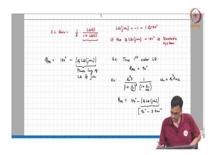
Alright. So, let us do some simple examples, a true first order system. What is the phase margin? What is the angle of the loop gain function? What is the phase lag of the loop gain function at the unity gain frequency if we had a true first order system? 90°. So, how much margin do we have for the loop to become unstable? We can add 90° before the loop becomes unstable.
