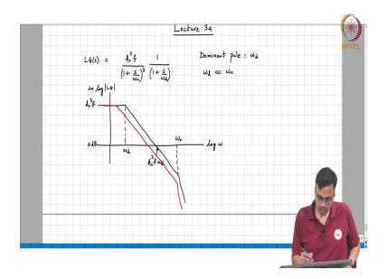
Good morning and welcome to Analog Electronic Circuits. This is lecture 34. So, in the last class, we were looking at trying to stabilize a high order system and for example, we had taken a system where the loop gain function had third order and recognized that the system is unstable for  $A_o^3 f \ge 8$ .
