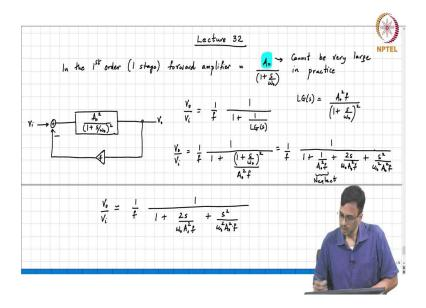
So, in the last class we basically looked at the stability of a 1<sup>st</sup> order closed loop system where the forward amplifier has got a single pole system. The nice thing about a single pole system is that the closed loop system is unconditionally stable right. And we also said that we also discovered that the unity gain bandwidth of the forward amplifier also happens to be the gain bandwidth product of the closed loop amplifier right.
