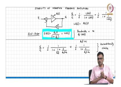
So, let us start with the simplest possible system you know, let us say a forward amplifier which is first order. So, A(s) is nothing but A<sub>o</sub>. It is DC gain, and there will be a single pole. So, let us call that  $s/\omega_o$ , in a common source amplifier that  $\omega_o$  will correspond to  $1/(Rs C_{gs} + 1 + C_{gd} A)$  etcetera, right, ok.
