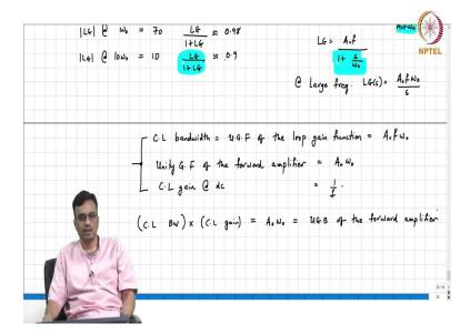
$A_o$   $\omega$ , alright. So, what is the closed loop gain at DC approximately? What is the closed loop DC gain?
