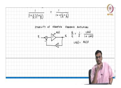
Alright, and you know before we start drawing circuits let us basically get back to our basic block diagram or the negative feedback loop we will do it at the block level. So, now we understand that this is not just a frequency independent gain this is a frequency dependent gain A(s) and the closed loop gain  $V_o/V_i$  is nothing but,
