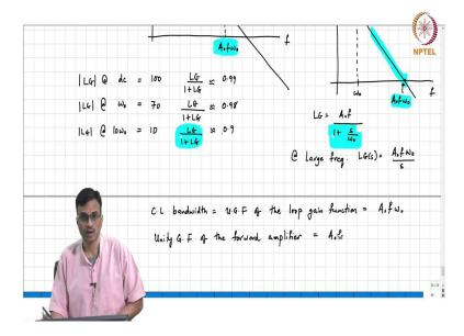
Ok. So, is the unity gain frequency of the loop gain function which is the same as  $A_o$  F  $\omega$ , ok. Next observation that I would like to make. What is the unity gain frequency of the forward amplifier?
