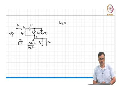
Then let us take a look at the other amplifiers that we have seen, namely the common drain. So, this is something that is  $v_i$ . This is  $R_L$  and let us say this is  $R_L$  and  $C_L$  this is  $C_{gs}$  and this is  $C_{gd}$  ok.
