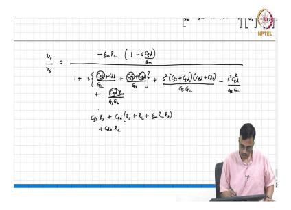
So, this is what I am going to simplify this further. This is  $C_{gd} + C_{gd}$ , let us say there is a  $C_{gs}$   $R_s$ ,  $+ C_{gd} R_s + R_L + g_m R_L R_s$ , ok. So, that basically takes care of these 3 terms,  $+ C_{db} R_L$ , ok. So, rather than do it this way, we can group terms with respect to  $R_s$ .
