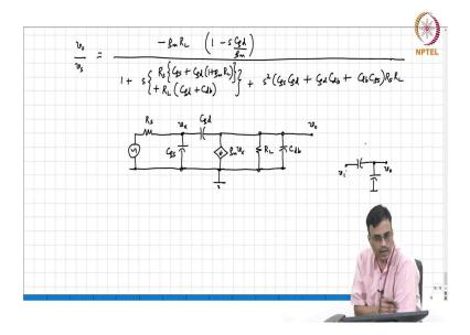
So, basically the point is that even though there are 3 energy storage elements, you have 3 of them connected in a loop. So, all the 3 you know capacitor voltages are not independent. And therefore, it is still a second order system, right. And in fact, how many energy storage elements are there here?
