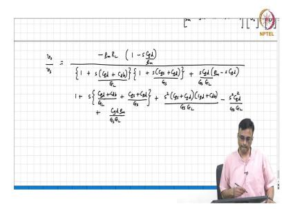
So, this is  $C_{gd}$   $g_m/G_s$   $G_L$ . I hope this is ok. Dimensionally it is consistent, ok. And then you have to subtract -  $s^2$   $C_{gd}^2/G_s$   $G_L$ . And God help us if you made a mistake, ok, alright.
