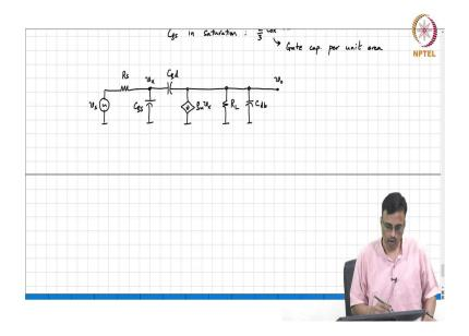
And the first I mean the biasing all remains the same, right. So, it is only may, it only makes sense to look at the incremental models of these amplifiers and see what effect the capacitances have on the performance of the amplifier. So, the first and simplest one is of course, the common source amplifier. I am going to draw only the equal, small signal equivalent.
