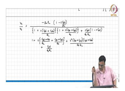
So, this gives us nothing but -  $g_m$   $R_L$  a numerator term which reduces to 1 when s=0 and a denominator term which also reduces to 1 when s=0. So, now let us simplify this stuff. So, this becomes 1+s  $((C_{gd}+C_{db})/G_L+(C_{gs}+C_{gd})/G_s)+s^2(C_{gs}+C_{gd})$   $(C_{gd}+C_{db})/G_s$   $G_L+C_{gd}/G_s$   $G_L$ . This is  $g_m$  - s  $C_d$  is it, but we removed the  $g_m$  common, is not it.
