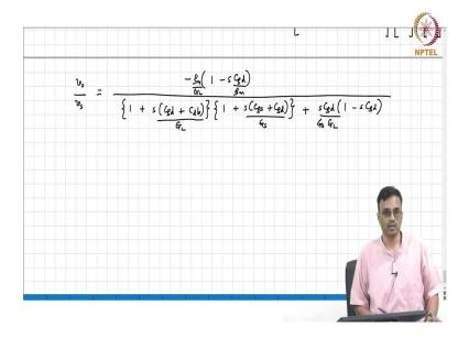
I just moved the  $g_m$  outside here. And I will move  $G_L$  out of the whole  $G_s$   $G_L$ , I will divide the denominator by  $G_s$   $G_L$ . So, this becomes  $1/G_L$ , this becomes  $1/G_s$ , this becomes  $G_s$   $G_L$ , ok. And therefore, the numerator I should get is  $1/G_L$ .
