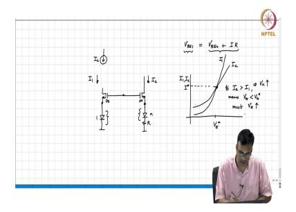
If you want the current, if you want to generate a ptat current, right, what happens eventually as we saw  $V_{BE1}$  must be equal to  $V_{BEn}$  +IR, correct? So, one way of finding that magic current  $V_T \ln(n)/R$  is to force the same current, ok. So, this is basically saying the voltage across this branch, remember that  $V_{BE1}$  is the voltage developed across the diode when the current is I.
