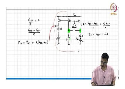
And then taking that current, pushing it to a larger resistor, right. Whichever amplifier you have seen, basically that is what is happening. So, the first job is to convert, you know,  $V_{BE1}$  -  $V_{BEn}$  into a current, alright. And before that, we said, we start off with converting  $V_{BE1}$  into a current, then we will figure out how to convert  $V_{BE1}$  -  $V_{BEn}$ .
