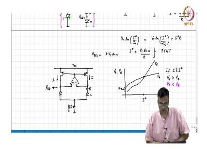
So, for very small values of I which will be greater I mean which will be greater  $V_A$  or  $V_B$ ?  $V_A$ . So,  $V_A$  will look like something like this  $V_B$ , for very small I will be this difference. For very small I will be  $V_T$  ln(n) because the drop across the resistor is very small. As you keep
