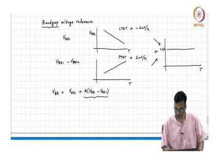
In the last class, we were looking at the basic idea behind the Bandgap voltage Reference. I will tell you why it is called the bandgap. So, the basic idea as you saw was to take a diode drop which we called  $V_{BE1}$  whose temperature coefficient is CTAT and roughly - 2 mV/K, right. And somehow generate a PTAT. If you generate +2 mV/K, if you add these 2, you get something which is independent of temperature, right.
