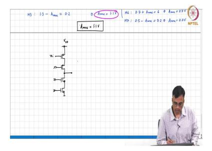
Let us take a look at the stage again, this is  $V_{DD}$ . This is appropriately biased, all these are bias voltages appropriately chosen that is what this means. So, the question is, what is the incremental gain? So, what do we do? We find the Norton equivalent correct.
