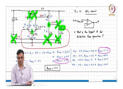
1 volt. What about M4? What is the highest the drain can go to? So, that is  $3.7 + A_{max}$  must be equal to?
