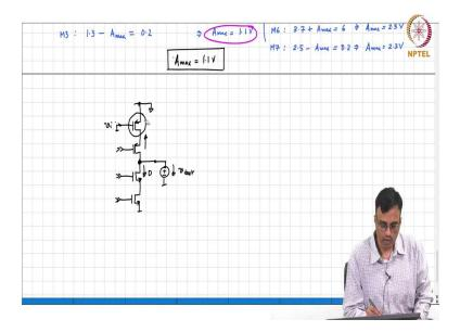
So, if we find the incremental equivalent this becomes ground to find the short circuit current, we connect  $v_i$  to incremental ground and measure the short circuit current. What is the short circuit current? This is  $v_i$ . What current is the incremental current flowing there?
