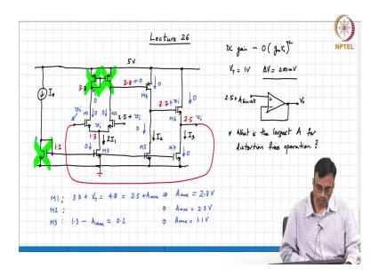
So, now you know which transistors do we need to worry about swing at all swing limits? Which of these transistors do we need to worry about? Ok. Let us start from the left with this guy. Well, the incremental voltage is 0 the incremental current is also 0. So, it does not change at all. So, that we are fine with. What about this chap here? We need to worry about it or not. Why? Why is there no incremental voltage across a transistor?
