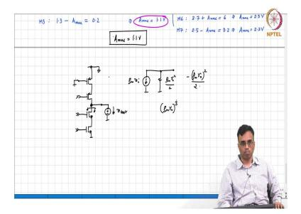
So, what is the output resistance? It is just the parallel combination of these two output resistances. Basically, it is roughly of the order of  $g_m r_o^2/2$  assuming all the  $g_m s$  and  $r_o s$  are the same. So, what is the gain that you get?
