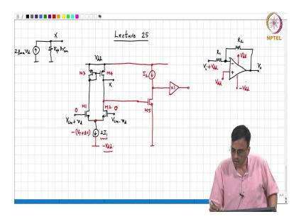
Alternatively, so, again we come back to our usual trick if we do not like negative supplies let us say this is -  $v_{dd}$ , what do we do? Add  $v_{dd}$  to all the nodes. So, in other words  $V_i$  instead of riding on ground right we will ride on  $v_{dd}$ . This will be  $v_{dd}$  this will be ground, and that will be  $v_{dd}$ ?
