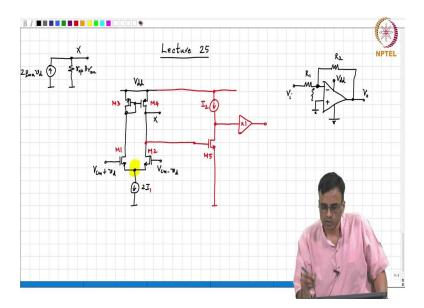
Now, the first thing that I would like to point out is the following and this has got to do with a lot of the circuit diagrams that you probably exposed to in the past and you see routinely in books and papers. And, for example, here is your common inverting amplifier which is  $V_o/V_i$  - $R_2/R_1$ , but clearly you do not expect the op-amp to work without any supplies, correct? So, what is the implication of drawing this picture?
