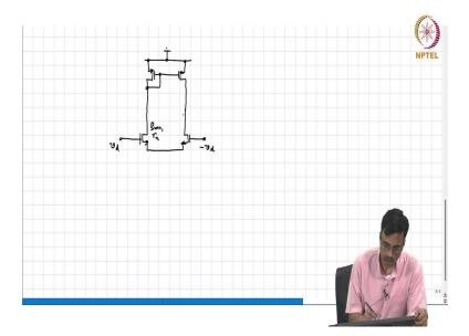
And this is I think the first time you are actually looking at circuits with more than 2 transistors, where both transistors are doing some work. In fact, we are looking at 4 transistors now. The incremental equivalent is all I am going to draw; we are going to go from there. Alright so that is ground. So, as usual I am going to this is  $v_d$ , this is  $v_d$  and so this is  $g_{mn}$ ,  $r_{on}$ , ok.
