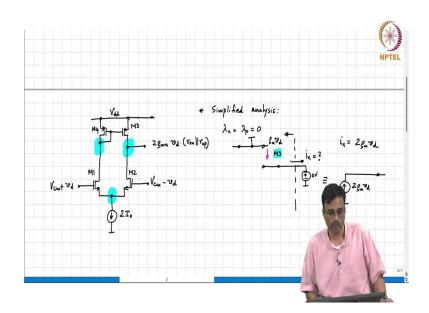
Therefore is nothing but 2  $g_{mn}$   $v_d$   $(r_{on}//r_{op})$ . Does it make sense? Ok so, that basically covers the differential pair with active load right. Now that I mean so, that finishes the discussion on the small signal properties of the differential pair.
