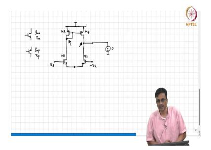
Because, this voltage is small, alright? What is this voltage? 0, because we have put the 0 voltage there to find the Norton equivalent, so this is small this is 0 this is small correct. So, for all practical purposes even though technically the circuit is not symmetric, right? If we assume that it is symmetric and then we go through the analysis.
