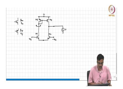
So, the NMOS transistors I am not going to mark it there, because it becomes very cluttered. So, this is  $g_{mn}$ ,  $r_{on}$  is the output resistance of the NMOS transistors, the PMOS transistor is  $g_{mp}$
