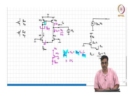
So, even though there is a resistance in the drain, because that resistance is small compared to yeah because it is small compared to the output resistance of M1, right. You basically have no influence on it. This is equivalent to saying exactly the same argument. I do not know if you
