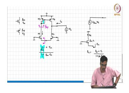
We inject, we apply a  $v_x$ , I will just write call it  $v_x$  and measure this is  $i_x$ , ok alright ok. Now, to do this let us mark down. So, what is the impedance looking in here approximately if  $1/g_{mp}$ , correct? Ok. So, what is it exactly?
