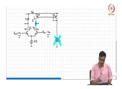
So, somebody suggested a current mirror, ok fine let us do that. If all the transistors are identical, what comment can I make about it? If all the transistors M1, M2, M3 and M4 are identical what comment I mean does it make sense or should I do this or basically what I meant to ask was are we ok with this current or is this is not correct?
