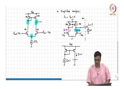
So, it is a current mirror after all, remember that in the let us say in the large signal picture in the if this current is I and this transistor is in saturation and  $\lambda$  is 0 what comment can you make about this current? If this changed by a small amount what comment can you make about the current in the mirror transistor?
