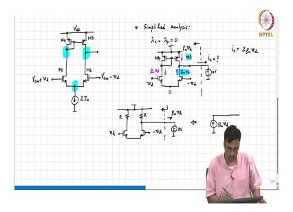
So, what is the short circuit current  $i_x$ ? 2  $g_m$   $v_d$  ok. Now how does this compare with the Norton I mean if we did the same thing with our regular differential pair where we had resistors. This is  $v_d$  this is minus  $v_d$  this is R this is R in the incremental picture this is grounded. If we found the Norton equivalent short circuit current of this guy. What would be the short circuit current?
