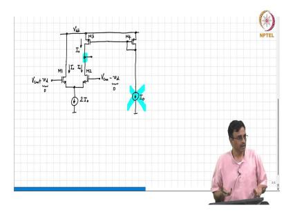
$V_{dd}$  alright. So, now, you can see that M1s drain current is just simply doing nothing; it is just simply connected to  $V_{dd}$  you might as well put it to work right. What does M4 need? And what is M1s drain current?
