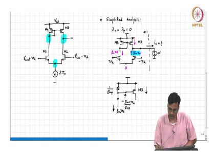
So, this is  $1/g_{mp}$  alright and let us call this  $g_{mn}$ . So, we separate the two alright and this voltage is connected there ok. So, what is this voltage therefore  $-g_{mn}/g_{mp}$   $v_d$  ok. So, what is M3 current through M3, what is the model for the PMOS transistor?
