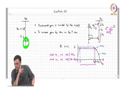
In the last class, we were discussing The Active Load and let me quickly go over that discussion. We were doing this in respect to a PMOS common source amplifier, but the discussion remains largely unchanged with an NMOS amplifier. So, the assumption is that this gate voltage is biased at a potential  $V_{\text{Go}}$ . The transistor is operating in saturation and carries a drain current  $I_{\text{D}}$   $I_{\text{o}}$ .
