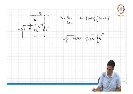
We can put in the drain directly. If you are concerned about DC current flowing through the load then you can as usual couple it to the capacitor. And so, the. So,  $V_G = V_{DD} R_2 / (R_1 + R_2)$ . So,  $V_{SG} = V_{DD} R_1 / (R_1 + R_2)$ .  $I_D$  therefore, is nothing but,
