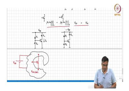
So, around let us take look at the let us say I had an NMOS transistor and a PMOS device and let us say for argument sake that  $\mu_n$   $C_{ox}$  W /L for the NMOS transistor is the same as  $\mu_P$   $C_{ox}$  W /L.
