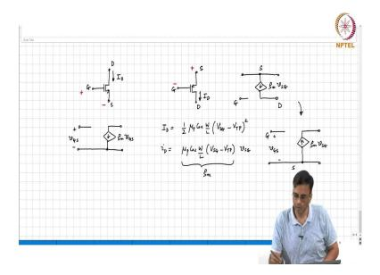
And so, the first thing we did when we saw the NMOS transistor was draw its, small signal equivalent and that was and this is  $g_m$   $V_{GS}$ . Now, the question is what do we do with the PMOS? Alright. So, remember the PMOS the drain current is  $I_D$  is nothing but in saturation is
