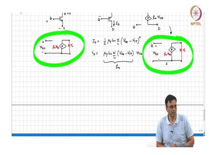
The consequence of that we already saw it was to simply add an output resistance  $r_o$ . This is  $g_m \ V_{GS}$  and similarly this is  $r_o$  this is  $g_m \ V_{GS}$ . Does it make sense? Ok. Now, that we have seen the basic what do you call incremental equivalent circuit; I mean we start making amplifiers like we did in the NMOS case. Let us start with the simplest one that is basically the common source amplifier.
