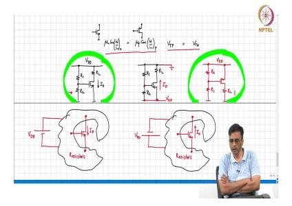
And as an example, you can see here. So, the source gate voltage in this case the gate source voltage was  $V_{DD}$   $R_2$  /(  $R_1+R_2$ ). Now the source gate voltages  $V_{DD}$   $R_2$ /(  $R_1+R_2$ ). So, earlier the current  $I_D$  was flowing downwards, now the current is flowing the same current  $I_D$  is flowing upwards alright, but of course, we do not like we do not like negative voltages first right. So, if we do not like negative voltages what do we do?
