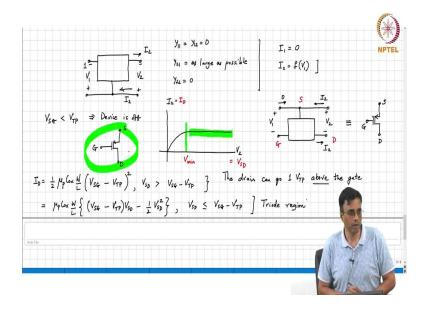
So,  $I_D$  turns out to be again first of all if  $V_{SG}$  right is less than some threshold quantity called  $V_T$  and now, earlier for the now we have two kinds of devices. Those are called the earlier devices called the NMOS transistors and their threshold is  $V_T$ . Now, since we have a PMOS transistor I mean this is what is called the PMOS transistor and therefore, to distinguish the thresholds of the two devices you know now you have a new subscript.
