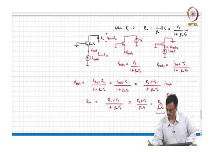
So, earlier we have seen what should happen when  $R_L$  is 0. When  $R_L$  is 0, what comment can you make about  $R_{in}$ ? We know this already. It is  $1/g_m$  parallel  $r_o$ , which is basically  $r_o/(1+g_m r_o)$ . Now, the question is what is the difference between this result and what we are looking for? Now, we have?
