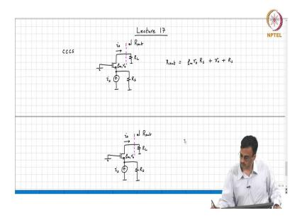
Alright, good morning, welcome to Analog Electronic Circuits this is lecture 17. In the last class, we were looking at the current controlled current source and we found that when the transistor has got a finite output resistance  $r_o$  the output resistance looking in. What is  $R_{out}$ ? It is basically  $g_m r_o R_s + r_o + R_s$ .
