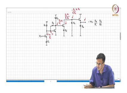
This is the incremental diagram, alright, ok. So, now, I mean the circuit looks pretty complicated, right. But you should be able to stare at it and tell me assuming that  $g_m$  is large, what is the output voltage?  $v - v_{in}$ .
