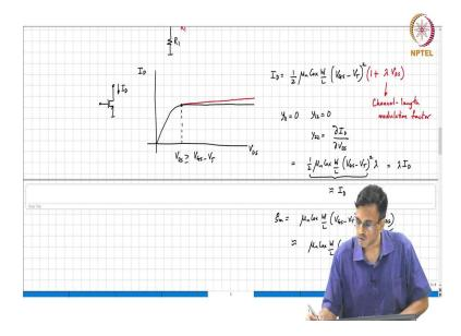
So, the next thing that I would like to talk about is, so far we assume that the IV characteristic of the transistor. So, the output characteristics of the transistor, right we assume to be the drain current  $I_D$ . In saturation, we assume that the current is independent of?
