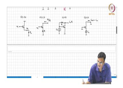
Alright. So, let us quickly summarize the 4 controlled sources. The first thing that we saw was the incremental voltage controlled voltage source and that is the common drain amplifier  $v_i$ ,  $v_o$ . Then, we saw the voltage controlled current source that is the transconductance amplifier. So, this is R, this is  $v_i$ . And this is; what is the trans conductance if  $g_m$  is very large? And, this current is  $v_i/R$ .
