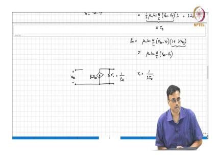
So, our model now is only slightly modified. So, this is  $g_m$  times  $V_{GS}$ . This is often called r o. It is also sometimes called  $g_{ds}$ . The conductance is called  $g_{ds}$ , right because it is between the drain and the source, right. And  $g_m$  expression is known,  $r_o = 1/\lambda \; I_D$ .
