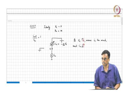
The last control source that we need to talk about is the Current Controlled Current Source. So, ideally, what comment can you make about the input resistance of a current controlled current source? Ideally, R<sub>i</sub> must be 0. What about the output resistance?
