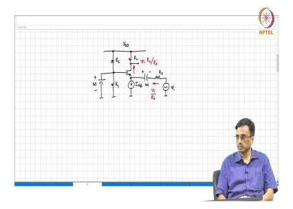
$I_{\text{ref}}$  is an open circuit in the incremental network, so that it will flow through the  $R_{\text{L}}$ . So, what comment can you make about the incremental voltage at the load?
