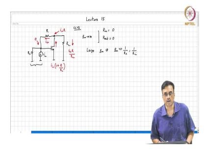
Good evening everybody and welcome to Analog Electronic Circuits, this is Lecture 15. In the last class we looked at the voltage controlled current. So, I mean current control voltage source where the incremental picture looked like this. This is  $i_n$ , this is  $R_L$  and if you assume that the current source has some internal resistance  $R_s$  then if  $g_m$  tends to infinity, what comment can we make about the input resistance?
