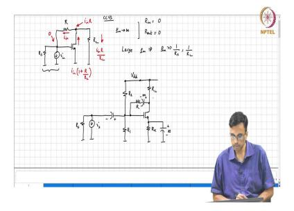
So, that is a transistor. So, what do we do with R? One way of doing it is to use an infinite capacitor to put R. What happens if I do not put a capacitor? Depending on the choice of  $R_1$ ,  $R_2$  and  $R_L$  a current could flow between through the resistor R and thereby disturb the operating point of the transistor, alright. So, this is basically you know perfectly working current controlled voltage source and you know nothing basically as we discussed the last time.
