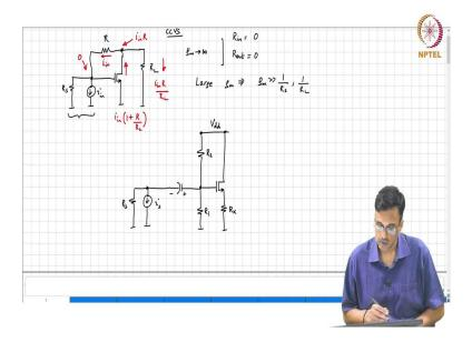
I am going to pick you know something for example, alright let me just pick something with gate voltage is constant, we measure at the source feedback at the source we use a poor man's current source and this is the  $V_{dd}$ , this is  $R_2$ , this is  $R_1$  and this is some  $R_X$ . And the job of  $R_X$  is to reduce the, why do we have  $R_X$  there?
