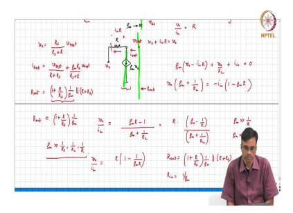
Now, if I remove  $R_L$  and if I want to find the input resistance, I mean let us do this quick, what is the input resistance?
