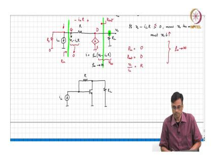
Infinite right. So, basically this current  $i = g_m (v_o - i_{in} R)$  and ideally  $g_m$  must tend to infinity alright. So, now can you identify the transistor?
