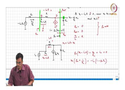
When the trans conductance is finite; so, let us call this  $v_x$  as  $g_m$   $v_x$ ; so, what is the current flowing through the resistor R? That current remains  $i_{in}$ , regardless of you knowing what happens because after all  $i_{in}$  the current source; so, what is the voltage drop across R is  $I_{in}$  R, alright; so, now, what is the only unknown or if you want to solve this network what will we do?
