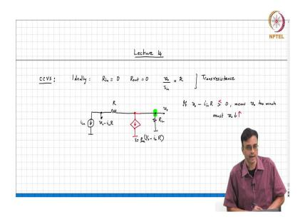
So, in the last class we were looking at how to realize the current control voltage source. Ideally of course, the input resistance must be 0, the output resistance must be 0 and the ratio of the output voltage to the input current must be some resistance R which is either called the transimpedance or the trans resistance. And the idea is very straightforward, we have an output voltage across load  $R_L$  and we want that to be equal to  $i_{in}$  R.
