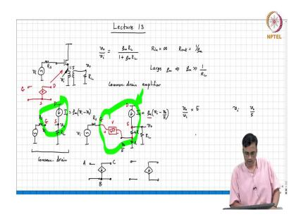
And this is a 1 : 5 transformer. So, by the definition of the transformer if this is  $v_o$  what is the input?
