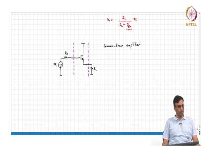
So, with this you know everything that we need to figure out about the amplifier is known. So, basically let me redraw the circuit, this is  $v_i$  this is  $R_s$  ok and as you can see which terminal of the transistor is common to both the input side and that is the input source as well as the load.
