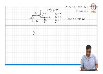
One is to simply compute  $v_o$  /  $v_i$  when  $g_m$  is finite and stare at that expression and figure out for what values of  $g_m$  that expression will tend to 1.
