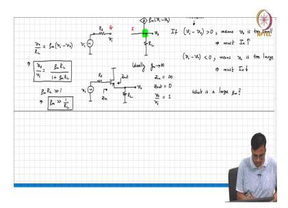
$g_m \ R_L$  must be much much greater than 1. Alright or equivalently the meaning of  $g_m$  a large  $g_m$  is that it is much much greater than  $1/R_L$ . So, to find output impedance, this is the gain with the finite  $g_m$ . What comment can we make about the output resistance? How will we figure it out?
