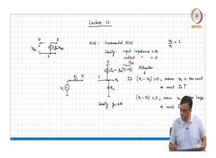
Good morning and welcome to Analog Electronic Circuits. This is Lecture 12. So, in the last class, we basically concluded by saying that we know that, in principle, the transconductance of a MOS transistor operating in saturation Actually, I think I have been using the notation "small v" capital  $G_S$  in principle because  $g_m$  can be, you know, as large as possible.
