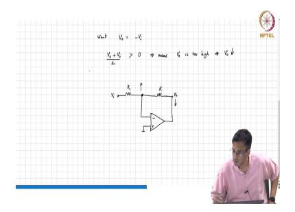
Alright, so now that you have the basic idea, let's get back to stabilising the bias of a transistor. As you know, we saw that we were using negative feedback to stabilise the bias current through the transistor. We saw two techniques already right, and the basic principle is the same for all of them: we measure the current in the transistor, compare it with the desired current, and tweak the  $V_{\rm gs}$  in the right direction.
