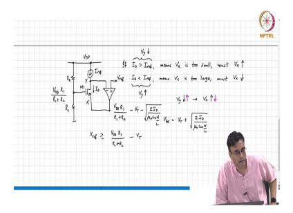
And go and vary the source voltage in the right direction now what is the right direction if V<sub>y</sub> goes up V<sub>x</sub> must go down. So, what are the signs of the OP amp?
