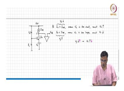
So,  $V_x$  therefore is a voltage that is controlled by the voltage  $V_y$ , alright and therefore it is a voltage-controlled voltage source between y and x. So,  $V_y$  you must compare it against some constant, let us call that,  $V_{ref}$  we only are interested in figuring out whether  $V_y$  is going up or going down. The only circumstance under which the potential of  $V_y$  does not change is when?
