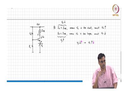
The drain, so you want to compare  $I_D$  and  $I_{ref}$  and let that node be y. So, in other words if  $I_D$  is greater than  $I_{ref}$  what will happen to the potential of node y? If  $I_D$  is greater than  $V_y$  it will
