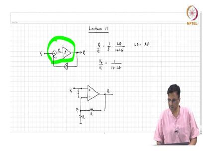
Alright people, good evening and welcome to Analog Electronic Circuits. This is lecture 11. So, in the last class we were looking at the basic negative feedback loop where you have a feedback block, forward amplifier, this is  $V_i$  this is  $V_o$ . And we set that,
