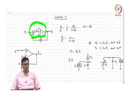
$I_{in}R$ . So, what will I do? So, what you are telling me therefore, is you generate  $I_{in}$  R somehow and the easy way to generate is simply pump in the current into a resistor then generate that resistor that  $I_{in}$  R. Tell me clearly what I should do this is  $V_x$  there is  $I_{in}$  R. Now what do we do? You put a voltmeter here that is a voltmeter. So, you have to put another voltmeter here. So basically, you measure you compare  $V_x$  with  $V_1$  which is?
