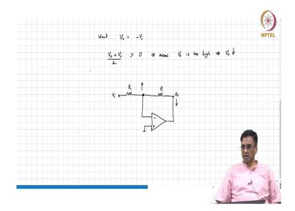
So, what I was saying was let us say we want  $V_o$  to be  $-V_i$ . So, what will we do? We will find  $V_o + V_i$  if  $V_o + V_i$  is greater than 0. What does it mean? It means  $V_0$  is too high and therefore,  $V_0$  must reduce and vice versa, is this clear? So, now, the question is  $V_0 + V_i$  greater than 0 is equivalent to saying  $(V_0 + V_i)/2$  is also greater than 0. So, how will you get  $(V_0 + V_i)/2$ ?
