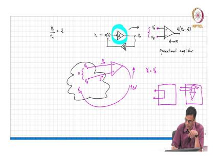
So, let us say we break the loop somewhere, say here and we apply a voltage in that direction. We apply a voltage  $\Delta V_i$  that direction. What comes back is a voltage going in the same direction at the other end of the loop, right. What does this mean?
