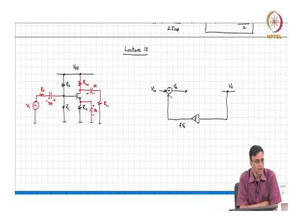
So, the source has to be incrementally grounded and we have to put the  $c_x$  there again. All these capacitors have to be infinite, alright. So, this gives you a common source amplifier. So, as we have seen over the last couple of lectures, the fundamental way of stabilizing something or making sure that something is a constant is basically through the use of negative feedback where the idea is you compare what you have with what you want.
