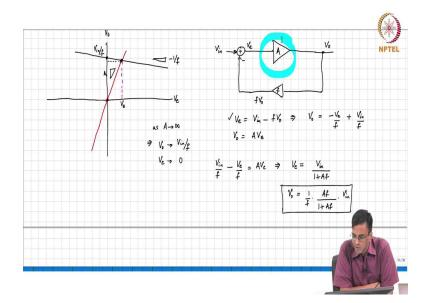
So, basically what you have is a voltage control voltage source. Let us assume some gain A. So, basically A must be positive because if  $V_e$  is positive, it means that  $V_o$  must be smaller than it should be, which basically means that it must be?
