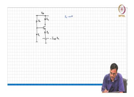
So, that is  $R_x$  and this voltage is minus  $I_{ref} R_x$ , alright. And what is the sanity check you know as  $R_x$  tends to infinity what happens? Well the impedance scene will go to infinity obviously, but the voltage is also going to infinity. So, that the current is maintained at?
