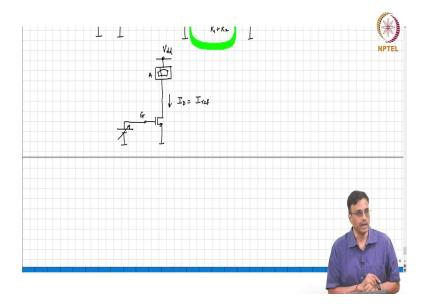
So, that the current in the drain is some desired current  $I_{ref}$ ? What would you do in principle? What would you do? So, basically what he is the principle is the following: that is you therefore at the gate you have to have a variable voltage. We apply some voltage source
