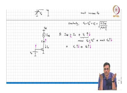
So, let us assume that the reference current is available as a current source. And we want to compare the reference current with the with  $I_D$ , the drain current of the transistor. So, how do we subtract these 2 currents, how do we get the difference between these 2 currents? You make you connect the two together and this is  $I_D$ .
