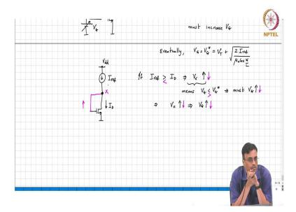
So, in steady state therefore, when the  $I_{ref}$  will be exactly equal to  $I_D$  and therefore the voltage developed at the gate is exactly that needed to make sure that the current in the drain is equal to  $I_{ref}$  irrespective of the properties of the transistor. Does it make sense people? Alright.
