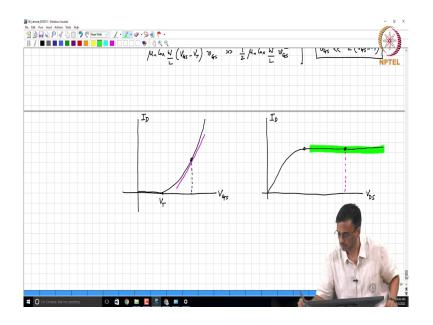
Let me go back to  $V_{GS}$ . If I plot the drain current as a function of gate source voltage in saturation, what curve will I get?
