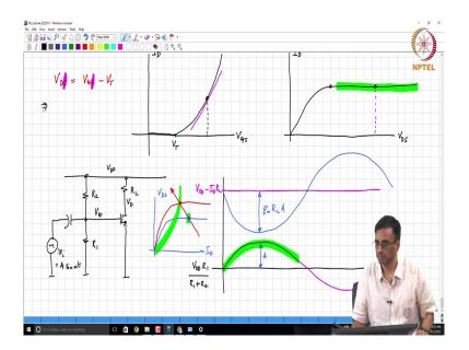
So, coming back to our common source amplifier. Now, this is  $R_1$ , this is  $R_2$ . Let me take the simplest possible one. So, I will put  $R_L$  here, this is  $V_{DD}$ . These are infinite capacitor we do not worry about it at this point simply because we already know what constitutes an infinite capacitor.
