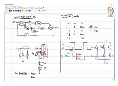
So, this is hybrid PLL, analog/digital, you want to write it, you can write it like this analog/digital PLL. So, here, we had PFD, the implementation of the PFD we have seen and then you had this feedback path from here. The PFD output goes to a DAC which I call as proportional path DAC or PDAC. The output of the PDAC goes to the oscillator and this I have been using a current controlled oscillator, for example.
