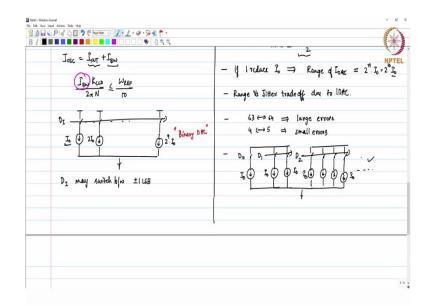
So, we will only look at IDAC and the current controlled oscillator. So, what we have here is a large number of bits coming from the digital accumulator going to a current DAC, this current DAC directly controlling the current in the oscillator or you can say the frequency of the oscillator. So, here I will call this as  $I_{INT}$ . So, now converting from  $D_I$  to your IDAC, the thing is that the total current which is required for the oscillator to oscillate at a given frequency in our case.
