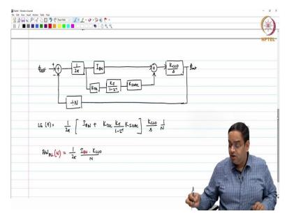
Now, similarly, what we are going to have here is the gain is here  $I_{BW}$  because that is the change by which the output current changes. So, we have this phase error, gain  $\frac{1}{2\pi}$  and from here it changes, you have this  $I_{BW}$ , this goes to your VCO but the VCO has the other factor also coming in from the integral path.
