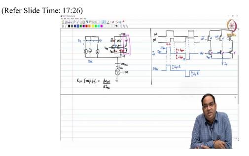
If you recall your voltage control  $\Delta V_{ctrl}$ , let me just put it back here, your  $\Delta V_{ctrl}$  because of the proportional path was in this case it would have been  $I_{CP}R$  and this would have been 0 and this case would have been  $-I_{CP}R$  whatever your charge-pump current is, that was the proportional path gain, this is the voltage and  $I_{CP}RK_{VCO}$  gave you the change in the output frequency.
