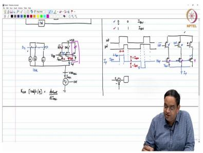
So, I will just draw the small signal model of the PFD now which has this phase error, + and -, the phase error you have if you look at the average current which flows out of this proportional DAC, that is going to be  $\frac{I_{BW}}{2\pi}$  with respect to the phase error. This is the same thing which you had in case of your PFD output with  $I_{CP}R$ .
