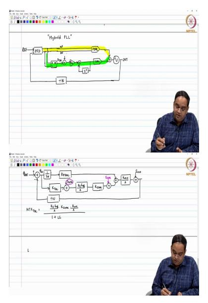
So, if I do that, let us bring this here. So, as I said that the minimum gain which I can have for the quantization noise from the proportional path, that is zero. So, I just removed the path altogether, make it zero. What is the big deal? Well, if I do this, I have two integrators in the path and when I have two integrators in the path, then it will also become a problem, the loop is not stable.
