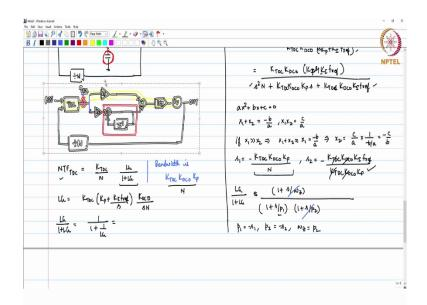
So, now, we would like to do something which helps us to reduce the effect of the quantization noise of the TDC. So, then we recall that in analog PLL, we did not have any quantization noise while measuring the phase error while here it has become a serious challenge. So, let us just compare the two. Analog PLL, when we had PFD, at that time the output of the PFD goes to charge-pump, charge-pump output goes to an analog loop filter like this.
