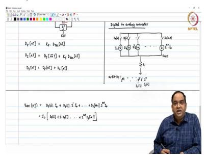
So, let me just try to show you one particular example of this m bit digital-to-analog converter. So, let us say these m bits are converted to control voltage using current sources. So, I am using current source like this and all these current sources are because this is just a simple implementation, you can do it in many different ways and all these current sources, they go to a resistor R. This current source I am because this is a m-bit number.
