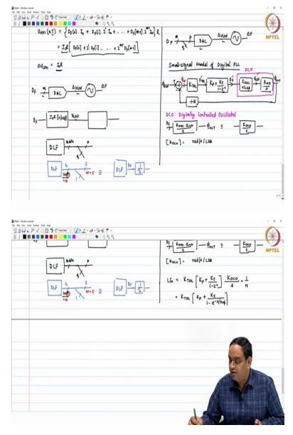
So, this can be written as, by the way if you look at it, this is nothing but the decimal equivalent of your digital loop filter output. So, whatever your digital loop filter output you have, so, your voltage which you are seeing here, your voltage is changing with  $\Delta V_{ctrl} = I_0 R$ . So, the control voltage is actually changing in steps of  $I_0 R$ , whatever you are using.
