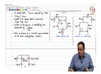
So, small signal model of the amplifier will be simply further left and Opamp with PMOS load is going to be this. There is no input, you are only looking at, so, let me just do it this way. It is a more ideal block, I am just rejecting right now or not including the  $r_{ds}$ . Let us just look at this, so, this is what you have and you are applying supply noise here which is vdd, small signal vdd, this is your V-tail node.
