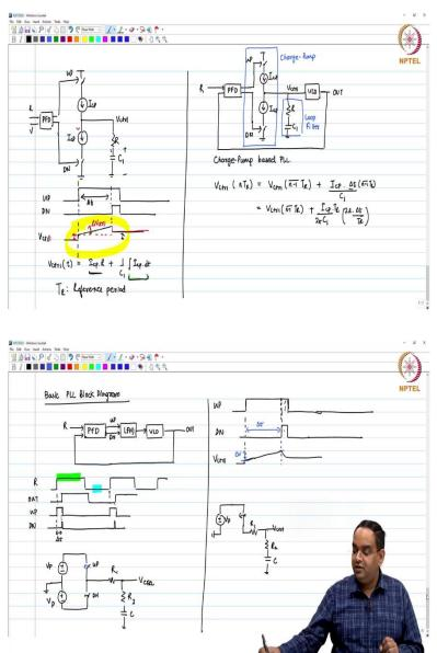
In contrast, you have a current based implementation where you again use two switches with two current sources like this. So, you have this switch controlled by UP, this switch controlled by DN, both the current sources are equal, and this is getting connected to the loop filter. Why am I using this loop filter? We will see it later but assume that this is the loop filter which we have right now.
