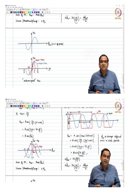
So, when we plot  $V_{PD}$  versus the phase error with respect to output phase, we see that it is sinusoidal. This is going to be like this. If you plot the same thing with respect to the timing error, I am not plotting with respect to the phase error, I plot with respect to  $\Delta t$ . If I plot with respect to  $\Delta t$ , then this value is  $\frac{T}{2}$  and this value is  $-\frac{T}{2}$ .
